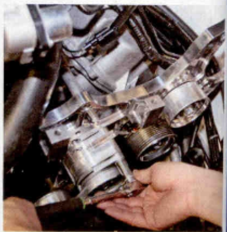
▲ With two of the four stand-offs mounted on the pulleys, Abe can now install the main bracket. It's one of the key components in the kit because it provides a rigid base for the supercharger to mount. The bracket is precision machined from 6061 T6 aluminum, and it's pocketed for lighter weight and rigidity.
