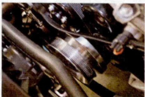
▲ Abe moves back under the hood to remove the factory serpentine belt and harmonic damper. A new two-piece billet damper is installed so that a second belt can drive the supercharger.
