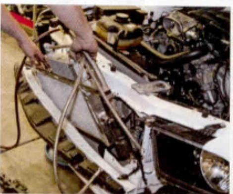
▲ The kit comes with a preassembled heat exchanger and oil cooler assembly. It's temporarily mounted
