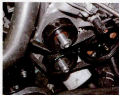
▲ Two billet stand-offs are installed onto two factory pulleys. This allows the main billet blower/pulley bracket to be mounted.
