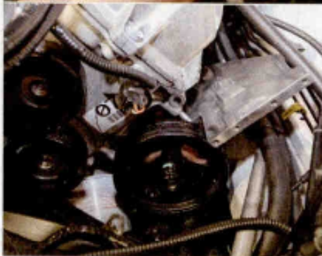
▲ An aluminum bracket to support the main billet blower/pulley bracket needs to be mounted behind the factory power-steering pump. Abe removes the pump and replaces a small factory spacer with the new bracket behind the pump using the stock bolts.
