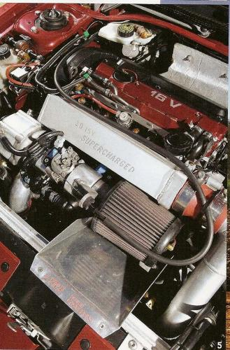
at the insides to ensure it wouldn't blow itself to pieces. Compression was the main issue; as standard the GTi-6 squeezes the air and fuel at a ratio of 10.8:1. 'I wanted serious power from the outset so I knew low compression was essential but I didn't fancy using a decompression plate between two head gaskets as I don't see the point in half doing things. Anyway reliability was a priority – I use it every day.'
