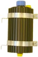
Place the oil canister with the cap **below** or **level** with the supercharger shaft. Use the bracket supplied in the oil set. Make sure the canister is placed upright. Leave the plastic plugs in place to prevent debris from entering the system
