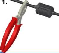
1. To avoid traction oil spilling into the engine compartment, use a hose clamp pliers to clamp the oil hose as close to the oil filter as possible on the oil canister side (filter inlet)
