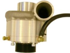
With the supercharger properly in place fit one end of the hose to the oil inlet using the banjo fitting and banjo bolt. Make sure to use a copper washer on each side of the banjo fitting to prevent leaks
