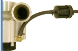
Now press the filter studs into the hose ends as shown and secure with hose clamps. Observe the flow direction of the filter! Following the same method, continue fitting the remaining parts of the oil system
